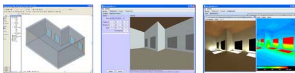
Figure 7 Existing design model from external CAD software (left). Automatic processing and population of missing values instantaneously and without user intervention (middle). Simulation results and analysis (right).
